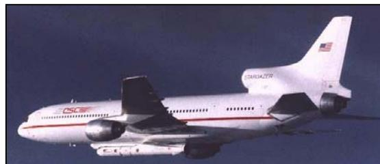
**Fig. 9-5. OSC's L-1011 Pegasus Launcher**
